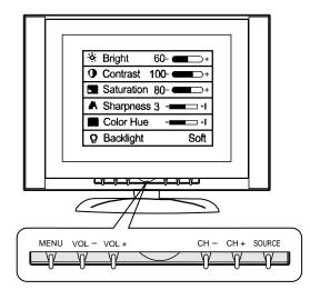
When there is correct input signal, press **MENU** button and **PC** menu appears. Use **CH+/-** to select item and **VOL+/-** to adjust
